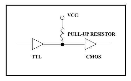
**Digital Input for Open / Short Switch Detection – A pull-up resistor must be connected, especially at long distance wiring, to ensure logic high input level.**
