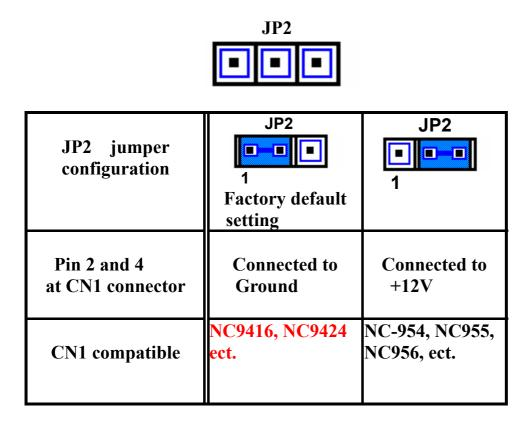
Jumpering PC +12V to CN1 connector allows the NC-911/910 to provide +12v power for direct relay driving voltage or input pull high voltage. Note that when using the NC-911/910 with standard Opto-22 interface panel board, pins 1 and 2 of JP2 jumper must be connected.
